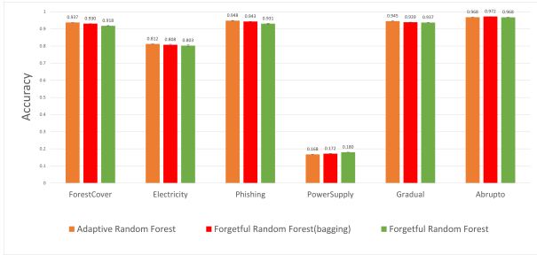
Figure 10: Accuracy of Random Forests: Without bagging, the Forgetful Random Forest is slightly less accurate (at most 2%) than the Adaptive Random Forest. With bagging, the Forgetful Random Forest has a similar accuracy to the Adaptive Random Forest
